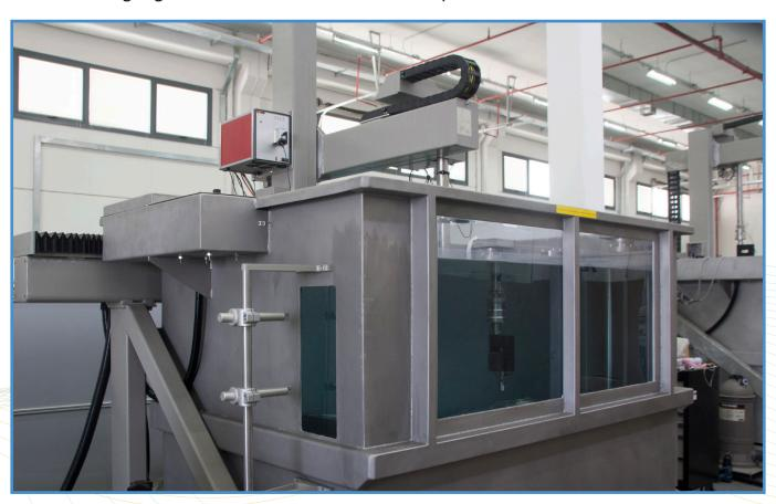
The LS-200 PA is based on the standard LS-200 Series scanner, which is equipped with a state-of-the-art fully parallel phased array instrument supporting linear, annular and matrix transducers, as well as a conventional high performance UT instrument.
