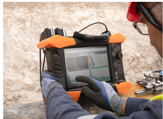
In-field inspection using M2M Gekko
