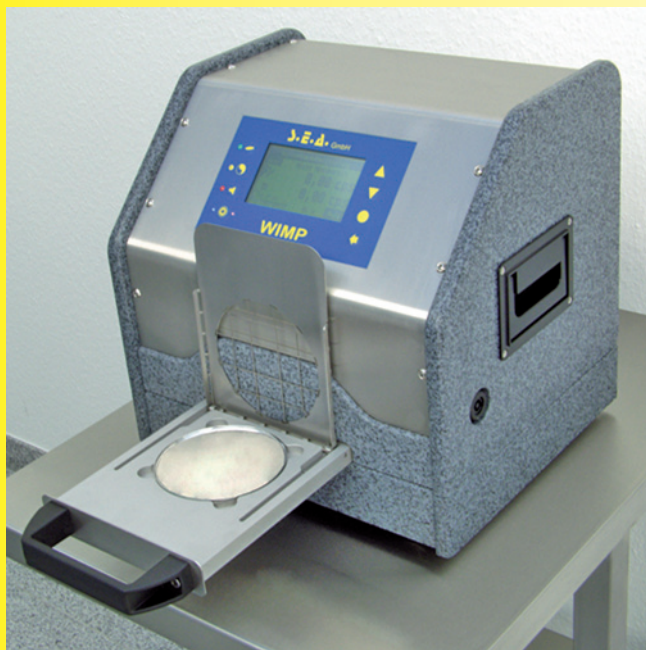
WIMP 120 C smear test counter with microcontroller
