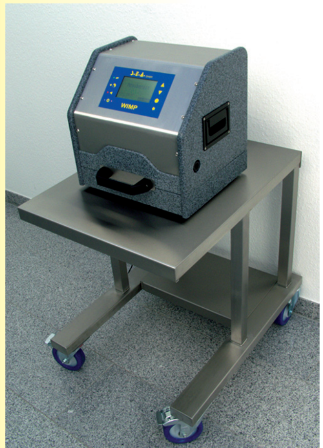
smear test counter on movable stainless steel table
