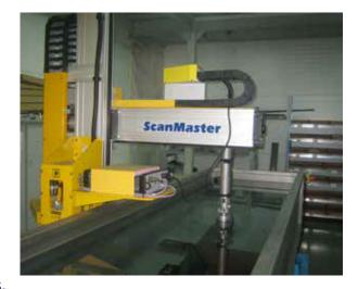
with detection of delaminations and porosity. Such areas can be inspected with or without mechanical surface tracking. The radii inspection can be performed either from the inside or from outside, depending on the accessibility, shape and size.
