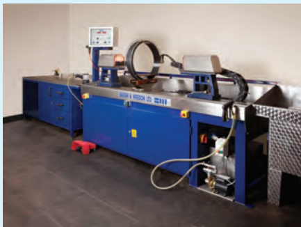
MAGAZON EBU MPI Benches ideal for testing large components
