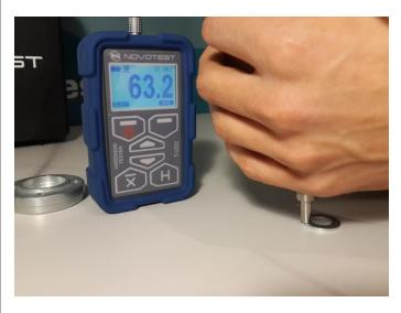
The ultrasonic contact impedance (**UCI**) probe is used for measuring the hardness of small items, objects with a thin wall, complex form, and to measure the hardness of surface hardened layers.
