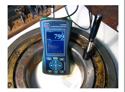
Device can be equipped with different types (D, DC, DL, C, D+15, E, G) of Leeb probe. Standard set of the device is included D type (universal) Leeb probe, other types by request.
