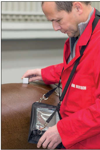
Mobile ultrasonic inspection with the ECHOGRAPH 1095 in the practical carrying case
